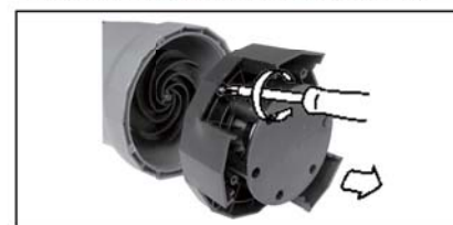
Figure C (Removing Base to clean Impeller)
